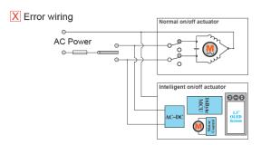
Note on wiring multiple actuators. Do not control AVA basic and Smart actuators in parallel using the same contactor.
