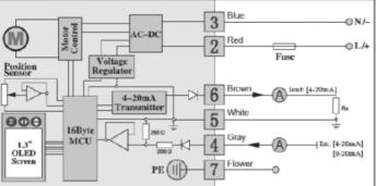
AVA actuators offer a 3 wire system with a permanent neutral on Blue, switchable Live between pins 2 (Red) and 1 (Black). Actuators are supplied with the a Pin connector as shown below as standard on model 20's. On model 60/110 the actuator has a terminal strip as standard.
