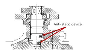
This device ensures the electrical continuity between ball, stem and body, required with flammable fluids.
